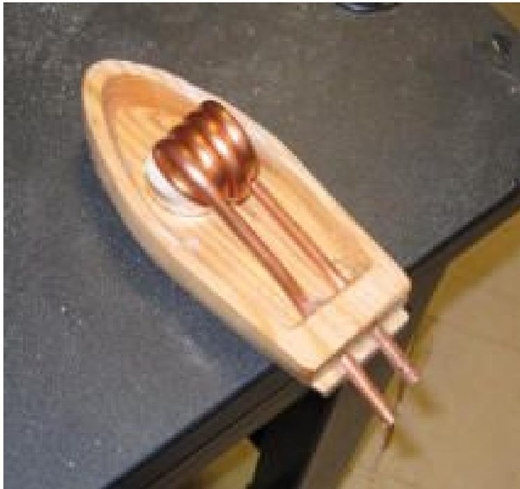
For my science fair project, I built a steam powered toy boat, or put-put boat. In the design, I varied the amount of area of copper tubing hit by the candle, to test its speed. Turns out that two coils is the best. Then, I tested it to see if it would fit to scale. Unfortunately, the boat I made was too big and couldn't float.
